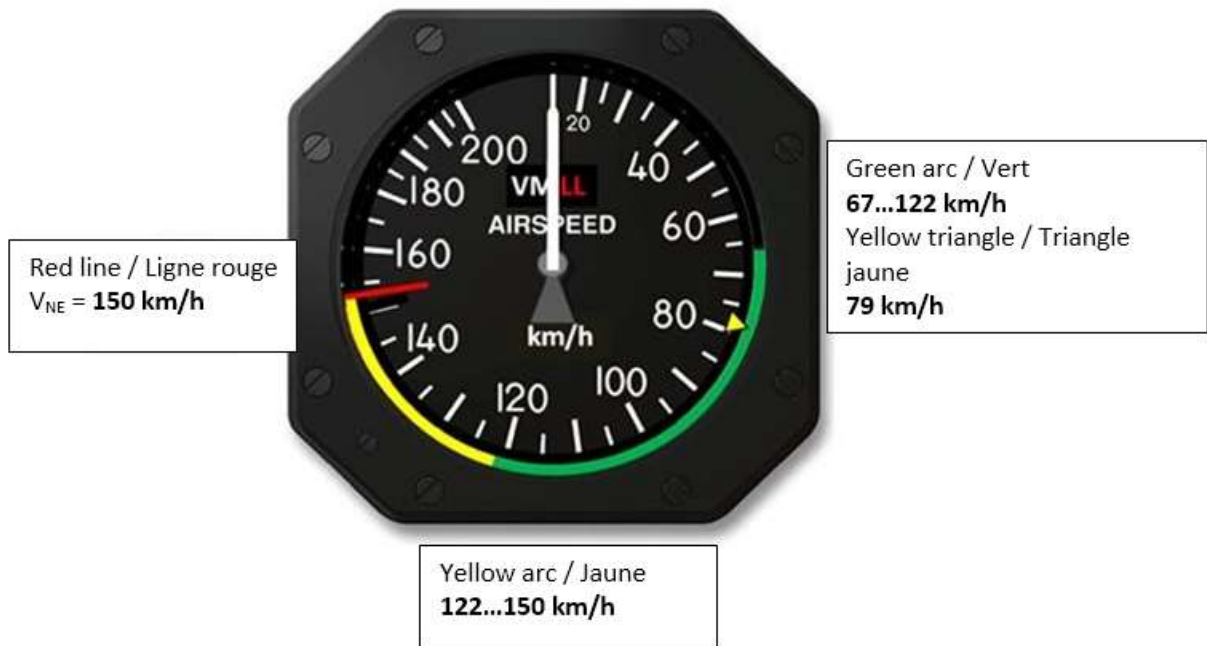
Airspeed Indicator with Coloured Arcs
